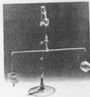
An instrument of the sort Galileo made: a delicate hydrostatic balance to find the density of precious objects on the principle of Archimedes.
